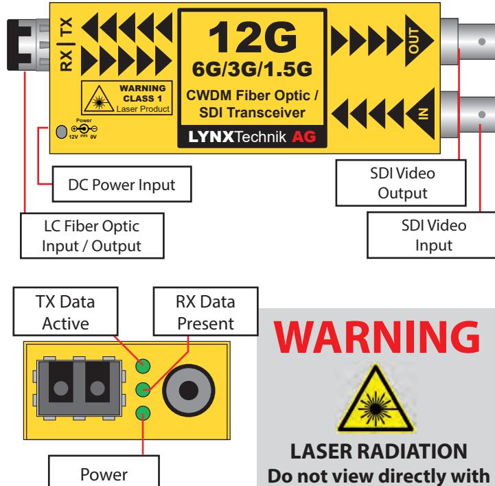
**WARNING:** Module laser is active as soon as power is connected, regardless of LED indication
