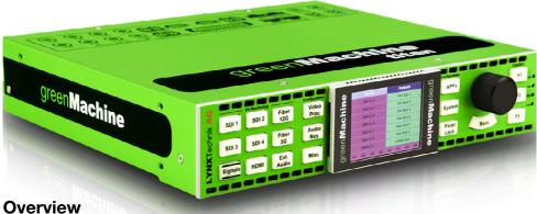
The current greenMachine titan comprises four 3G/HD/SD-SDI video channels or a single 4K/UHD video channel. It offers up to 12G processing support (3840 x 2160 @60 Hz) and provides the functionality to convert between single-link 4K video (12G) and guad-link 4K video (2SI; 4x3G).
