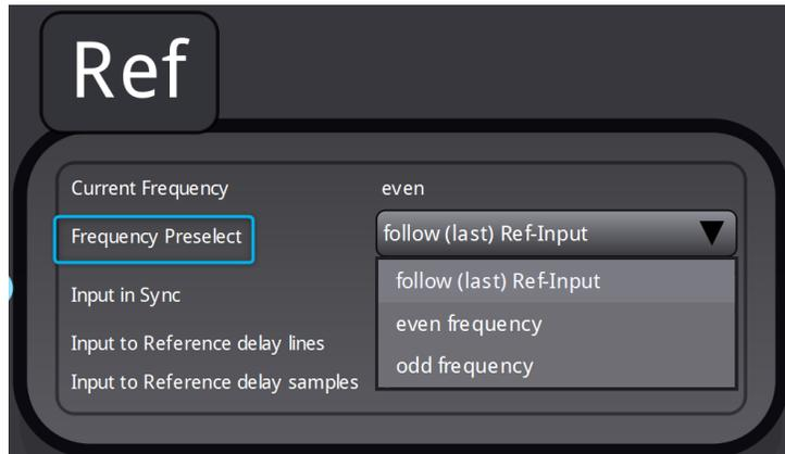
However, if the input reference signal changes, the video output may experience frame repetition, frame drops, or jitter to reconcile the mismatch while maintaining the locked frame rate. It is also possible for the synchronizer to configure the output frame rate based on the connected reference. This is the default setting. Possible settings are:
