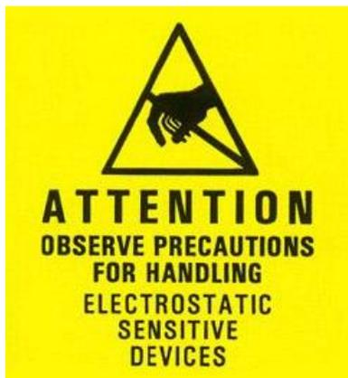
This product is static sensitive. Please use caution and use preventative measures to avoid static discharge that could damage the card module.
