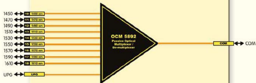
OCM 5892 - 9 Channel CWDM Optical Multiplexer
