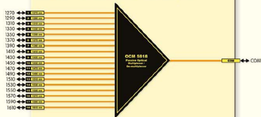
OCM 5818 - 18 Channel CWDM Optical Multiplexer
