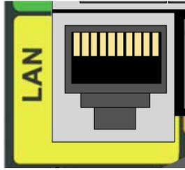
This is a standard RJ45 connection and is used to provide TCP/IP network control connectivity into a control system.
