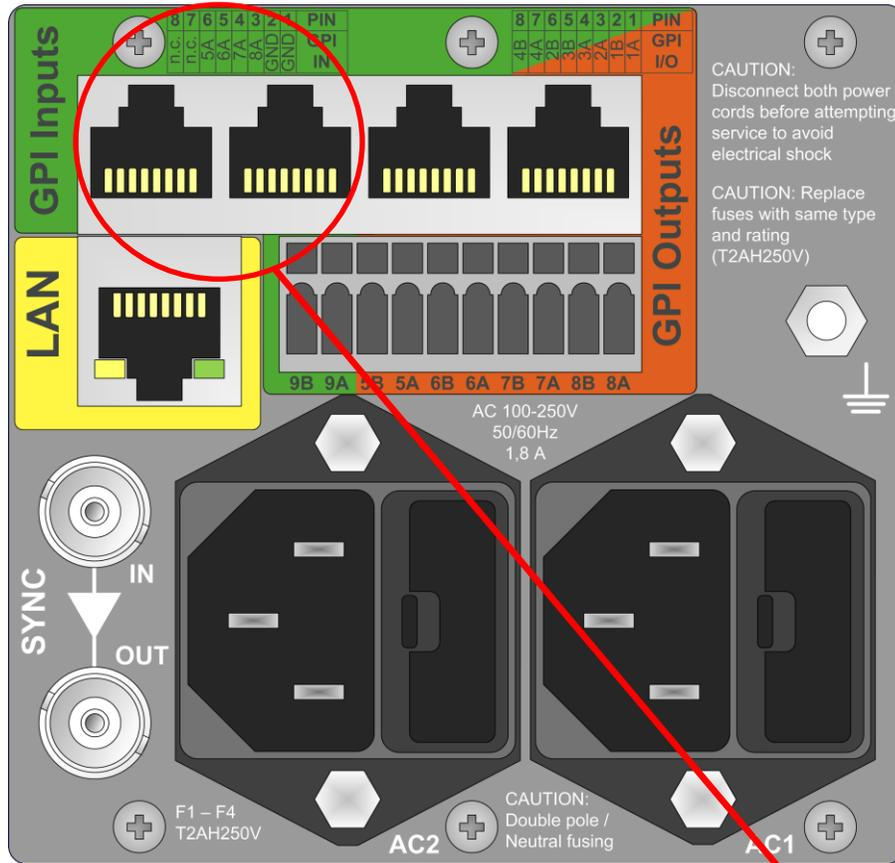
The two RJ45 connectors are looped through, so connections can be done through the one or the other connector. Pinning of the RJ45 connectors is according to TIA/EIA 568-B.
