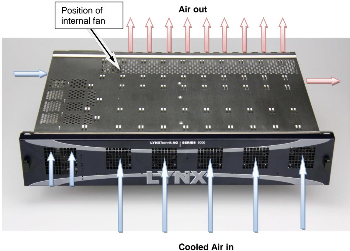
Additional ventilation holes are provided left and right of the rack frame to allow for some airflow if the front cover is open or removed. A fan in the back of the rack frame supports this additional airflow.
