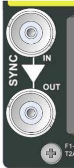
An external sync reference can be connected to the rack. An active loop through connection is provided with relay bypass in the event of a power failure.
