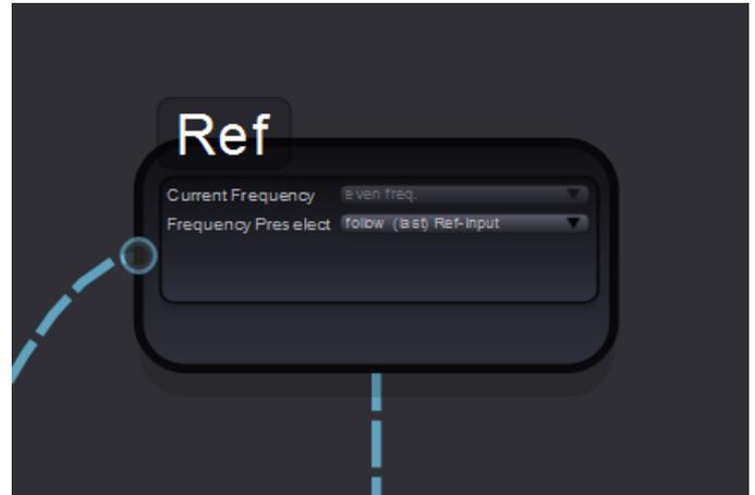
It is also possible for the synchronizer to configure the output frame rate based upon the connected reference. This is the default setting for the module. Possible settings are:
