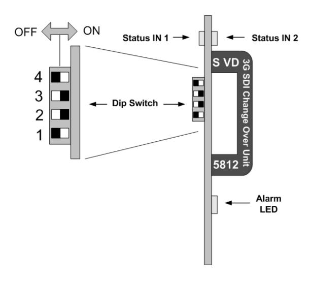
Figure 3 – Switch and LED locations
