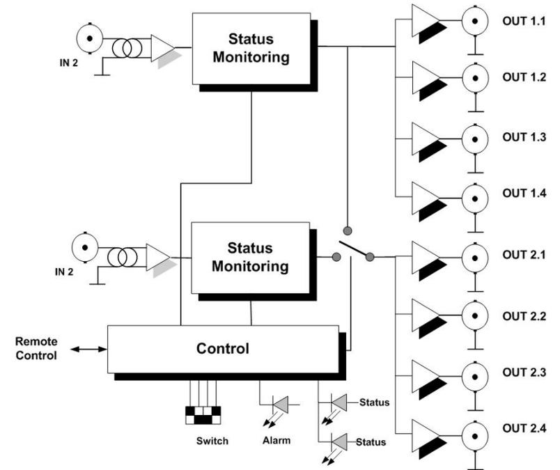
Figure 1.1- D AD 5220 WCB Functional Diagram
