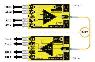
The fiber connection is made between each  ${\bf COM}$  port. The  ${\bf UPG}$  port is used to connect the OTR 1441 to add 4 more SDI channels, or connect a OBD 1510 E to add Ethernet , or OBD 1510 D to add Serial RS232 and GPI
