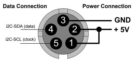
Male Connector (view looking into connector from front)
