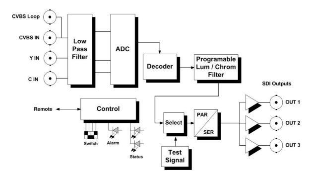
Figure 1- C AD 3100 Functional Diagram
